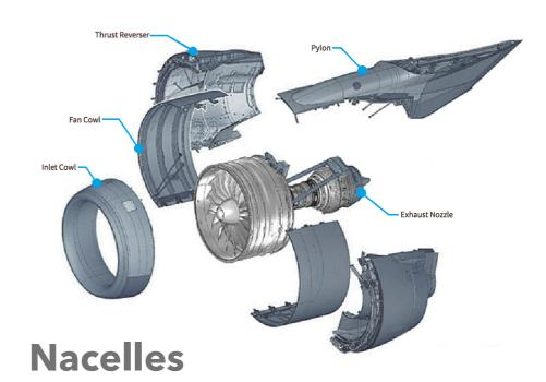
Specializing in Nacelle repairs, PCS has a dedicated Nacelle Division which can handle any requirement for your V2500, CFM, Trent, PW4000, RB211 and CF6 inlet cowls, fan cowls, reversers, sleeves, and doors.
